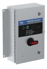
PQ480 is a high-performance, robust surge protective device (SPD) with advanced features, protecting your facility's electrical equipment from damaging electrical power surges due to lightning; utility power generation/distribution systems; and inductive load switching equipment within your facility. PQ480 is intended for Service Entrance and large equipment applications, incorporating integral rotary disconnect switch.
